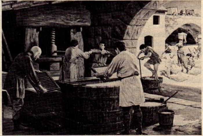
17th century papermaking in Fabriano, Italy. At the far left can be seen the coucoucher, while the vatman stands in front of the vat forming sheets of paper with a hand hold.
