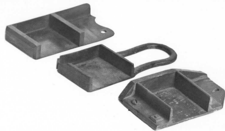
Newspaper composition sticks, 13 pica. (top to bot.) Brass, cast iron, and wood and metal. Nineteenth century.
